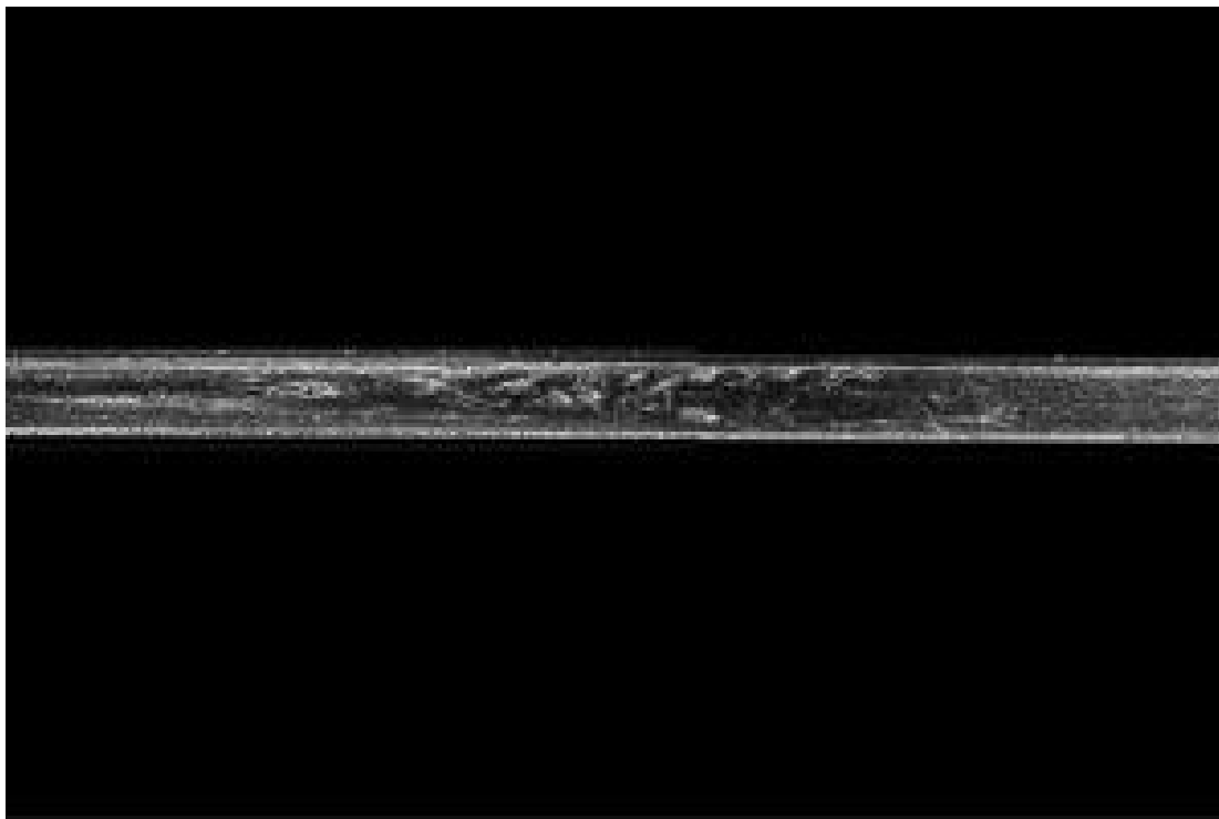
A turbulent eddy flowing through a thin glass pipe. The flow is laminar in front of and behind the eddy. (Credit: MPIDS)
